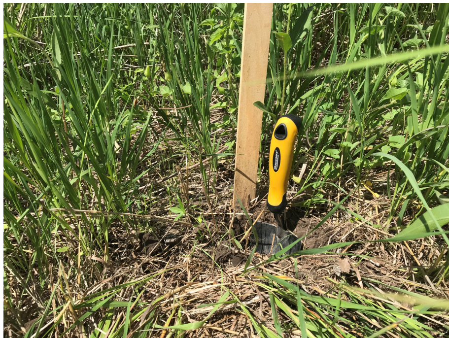
Figure 2: Composite soil sampling location observed with a garden trowel for scale. To avoid cross contamination, a different trowel was used for each composite sample, and discarded after.
