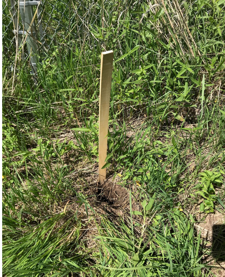
Figure 3: Composite soil samples were collected to depths of 0-0.5'. The samples were collected as close to the surveyed stakes as possible.
